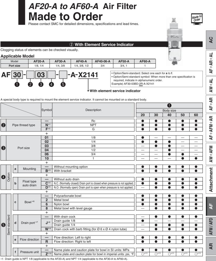
The auto drain port comes with Ø 3/8" One-touch fitting (applicable to the AF30-A to AF60-A). \*2 Drain guide is G 1/8 (applicable to the AF20-A) and G 1/4 (applicable to the AF30-A to AF60-A).
