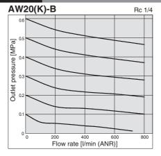
Condition: Inlet pressure of 0.7 MPa
