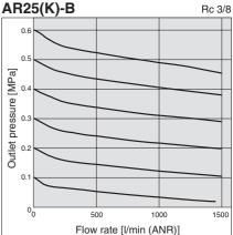
Condition: Inlet pressure of 0.7 MPa
