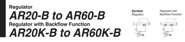
• With the backflow function, it incorporates a mechanism to exhaust the air pressure in the outlet side reliably and quickly.
