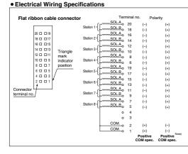
As the standard electrical wiring specifications, double wiring (connected to SOL. A and SOL. B) is adopted for the internal wiring of each station for 8 stations or less, regardless of valve and option types.
