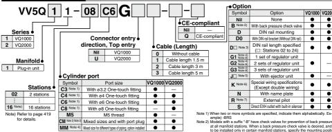
Note 1) Insert "L" (Top ported) or "B" (Bottom ported) for elbow type Example) B6 (Bottom ported elbow with ø6 One-touch fitting)
