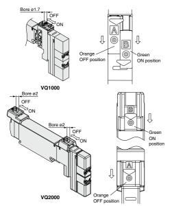
The manual override is locked by sliding it all the way to the pilot valve side (ON side) with a small flat head screwdriver or finger. Slide it to the fitting side (OFF side) to release it. In addition, it can also be used as a push type by using a screwdriver, etc., of ø1.7 or less. (ø2 or less for VQ2000).
