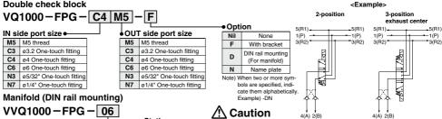
When ordering a double check block, or der the DIN rail mounting [-D].
