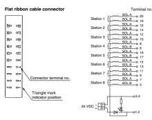
As the standard electrical wiring specifications, double wiring (connected to SOL. A and SOL. B) is adopted for the internal wiring of each station for 8 stations or less, regardless of valve and option types. Mixed single and double wiring is available as semi-standard. Refer to page 419 for
