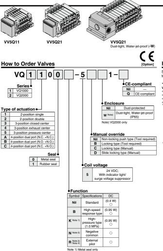
Note 2) For external pilot and negative common specifications, refer to "Semi-standard" on pages 419
