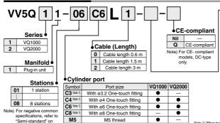
MM Note 4) Mixed size for different types of piping, option installed Note 1) Insert "L" (Top ported) or "B" (Bottom ported) for elbow type. Example) B6 (Bottom ported elbow with ø6 One-touch fitting)
