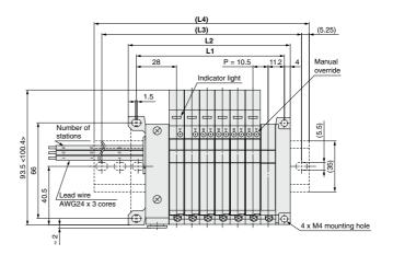
C8 [3(R) EXH port] C8: ø8 One-touch fitting DIN rail clamp screw 40.7 22 .... (7.5) (12) 20 C8 [1(P) SUP port] 33.3 P = 10.5 C8: ø8 One-touch fitting C3, C4, C6, M5 [4(A), 2(B) port] C3: ø3.2 One-touch fitting
